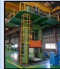
Backward extrusion preform
