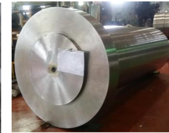
One piece main cylinder(Solid without welding)
