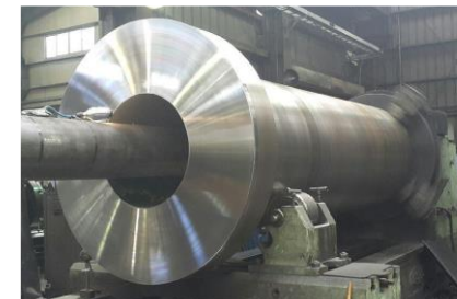
One piece main cylinder(Solid without welding)
